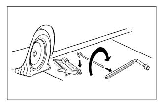
Insert the hooked end of the extension handle through the jack and the flat end through the wheel wrench.
